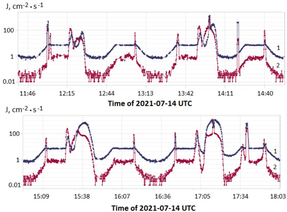
Fig. 7. Time variation of the count rate for electrons with energy > 300 keV (red curve) and for gamma-quanta (dark blue curve), recorded in the monitor mode of the *DeCoR* instrument operated on-board *Norbi* satellite on July 14, 2021.
