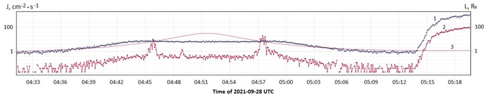
Fig. 8. Time variation of the count rate for electrons with energy  $E_i < 300 \text{ keV}$  (red curve), and gamma-quanta (dark blue curve), and L values (violet curve) recorded in the monitor mode of the DeCoR instrument operated on-board Norbi satellite on September 28, 2021.
