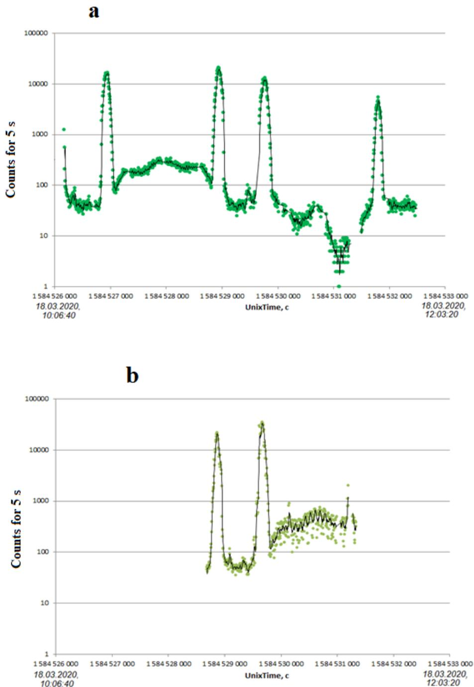
Fig. 6. Time variation of the count rate for electrons with energy  $\geq 300$  keV, recorded in the monitor mode of the DeCoR instrument operated on-board VDNH-80 satellite on March 18, 2020 (a), similar readings of the DeCoR instrument on-board AmurSat satellite (b).
