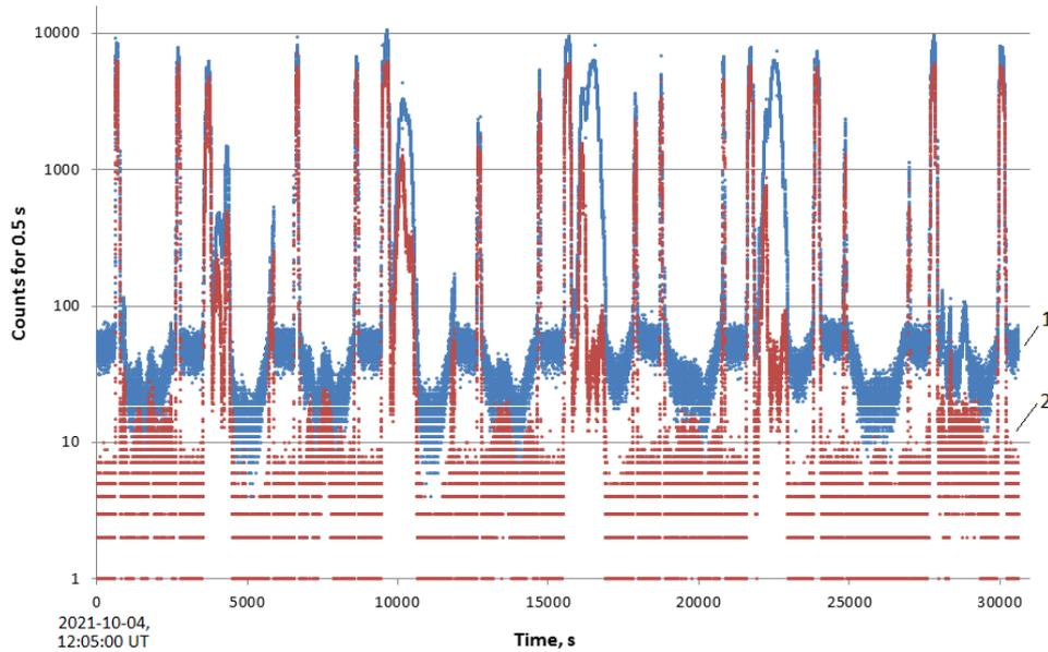
Fig. 9. Time variation of the count rate for electrons with energy  $> 300 \text{ keV}$  (red curve) and for gamma-quanta (dark blue curve) recorded in the monitor mode of the DeCoR detector on-board DEKART satellite on October 4, 2021.
