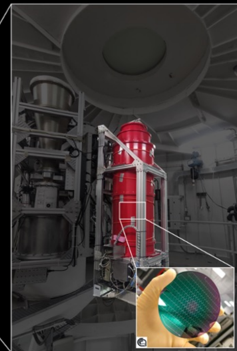
MISTRAL installed in the gregorian room of SRT and its detector array during fabrication
