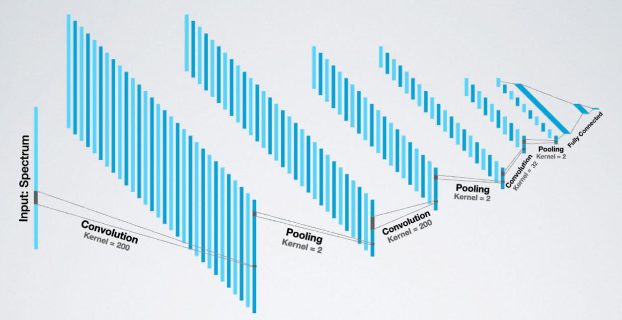
Structure of one dimensional CNN. The spectrum of quasar is input as a onedimensional array, which goes through the convolutional layer of kernel size = 200, 200, 32 respectively in order to search for the global and local pattern. The fully connected layers output the redshift.
