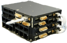
ICU : digital control laws, data conditioning
