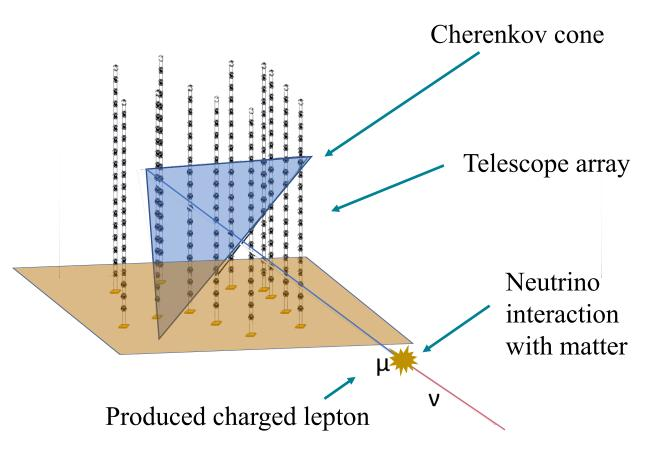
Time and position of photons to reconstruct the Cherenkov cone  $\rightarrow$  neutrino incoming direction
