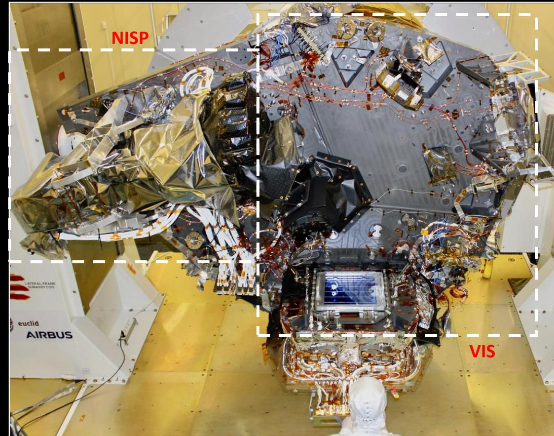
NISP and VIS integrated on the flight PLM baseplate
