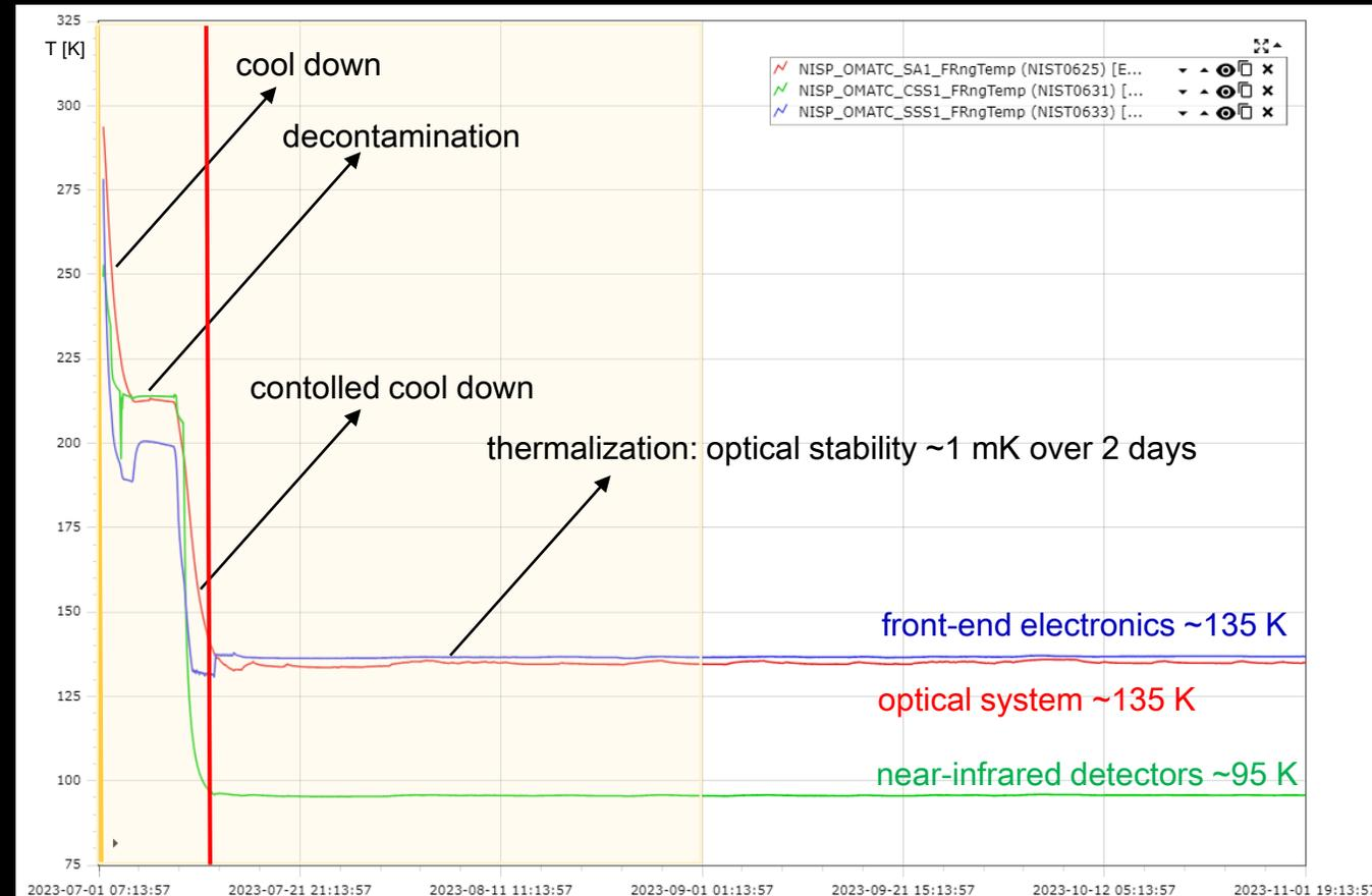
NI-temperature profile during early flight phases
