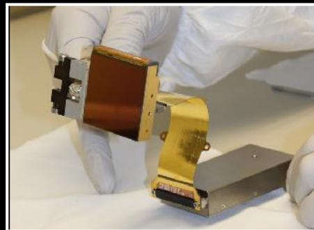
H2RG – flex cable – SIDECAR ASIC
