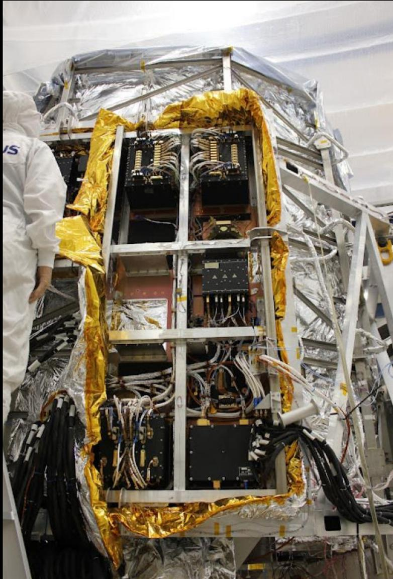
NI-WE is composed of 2 identical Data Processing Units (DPU) and 1 Instrument Control Units (ICU)
