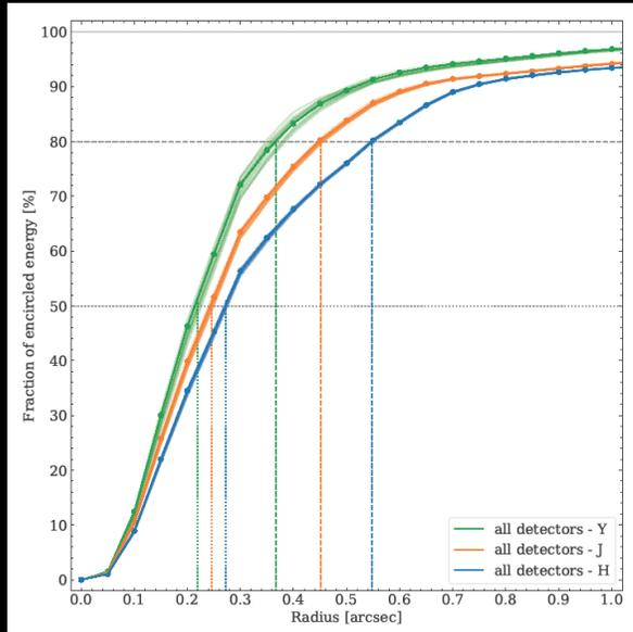
Modelled encircled energy (EE) of the NISP PSF in the 3 photometry channels from data acquired during the PV phase.
